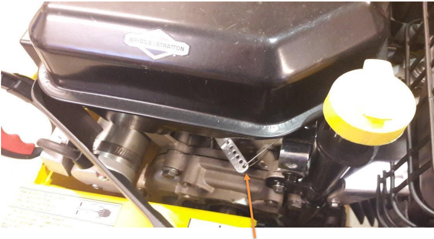
Picture 1. Open the engine side cover and raise engine rounds. Place the spring in position 6 (3600 r/min -> 4200 r/min). Add oil in the engine recommended amount, see B&S engine manual.
