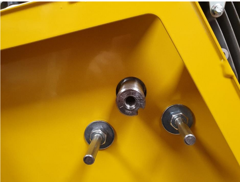
Picture 4. Make sure that the engine shaft is middle of the hole and tighten engine bolts.
