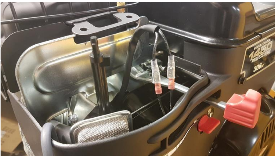
Picture 6. Push the ignition wires under engine side cover and make electrical connection like in the picture. Make sure, that wires are not too tight.
