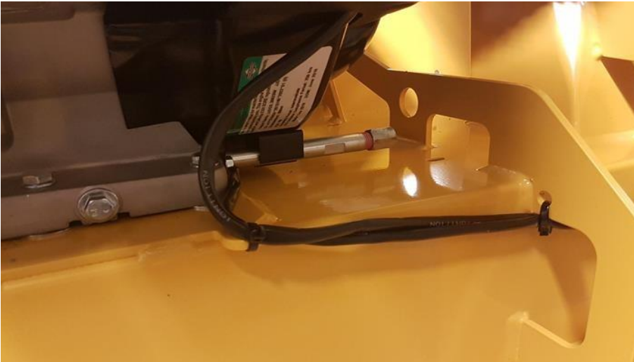
Picture 8. The correct way to install wirings. Notice that ignition wires are not too tight under cover.
