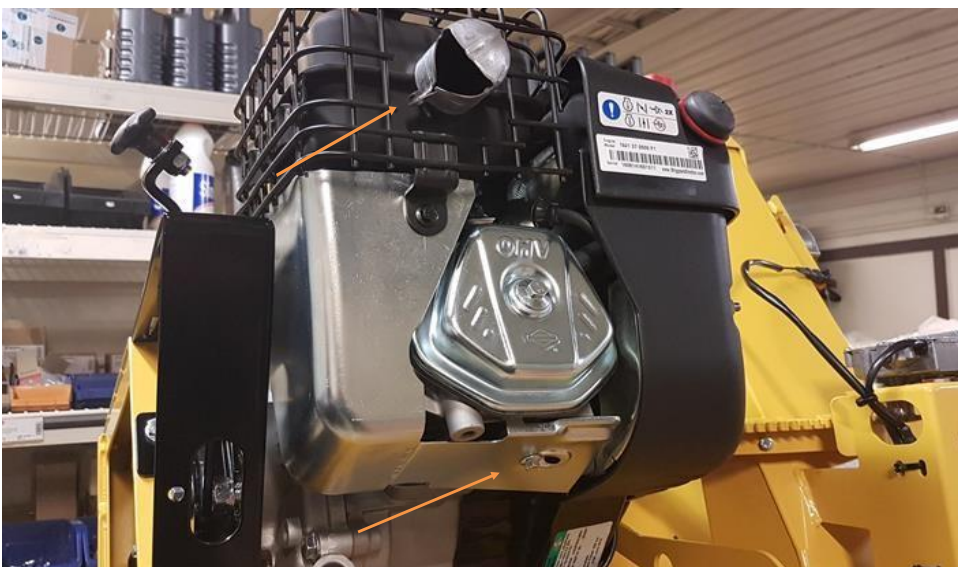
Picture 12. Install exhaust pipe like picture. Exhaust gases should blow about 45 degrees down-left. If the engine heat-cover hits against clutch frame, remove bottom bolt (picture) and drill 7mm hole near original hole. That moves heat-cover inner out of the clutch frame.
